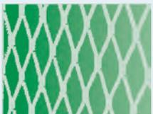
Expanded metal fences are very rigid (if correctly installed) and can be galvanised or polyester coated for longevity. They are difficult to cut through but repairs are likely to require whole panel replacement. Consideration should be given to potential livestock movements since the mesh tends to have sharp edges that could cause injury.
